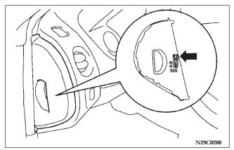
4. There is a fuse puller in the cover of the instrument panel (driver's side). Remove the fuse puller, clamp it on the fuse you wish to remove, and pull the fuse straight out from the fuse block. If the fuse is not blown, something else must be causing the problem; contact an authorized dealer to have the problem checked.
